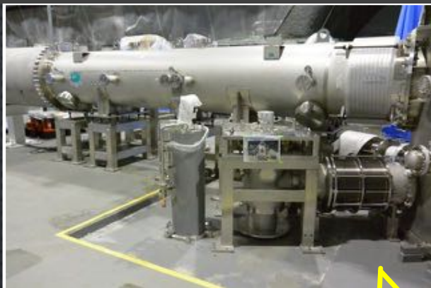
Ultra-small Vibration Cryocooler & Duct Shield
