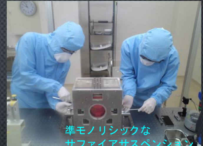
Semi-monolithic sapphire suspension
