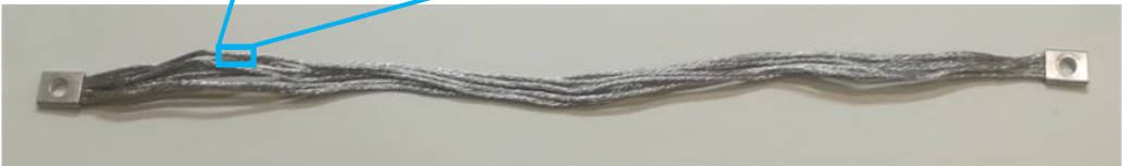
Stranded-cable type heat link ( \phi 0.15 mm \times 7 \times 7 \times 7)
