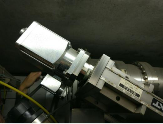
Close the "L angle" valve in between the turbo pump and the rotative pump
