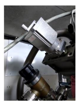
2. Turn off the connection between rotary pump and turbo pump
